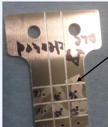
(A) Front side of the free-standing AAO mounted on a C-shaped Al-frame. (B) Experimental setup with target wheel and online imaging system used for laser focal spot optimization and target alignment. (C) Shadowgraph image of a 20 \mu\text{m} -thick AAO target. C. Gheorghiu et al., Frontiers in Physics, 2021
