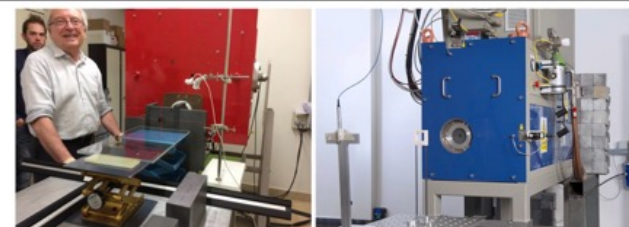
Kinetron PBM/Alcen Electron beam, 4.5 MeV energy Pulsed beam
