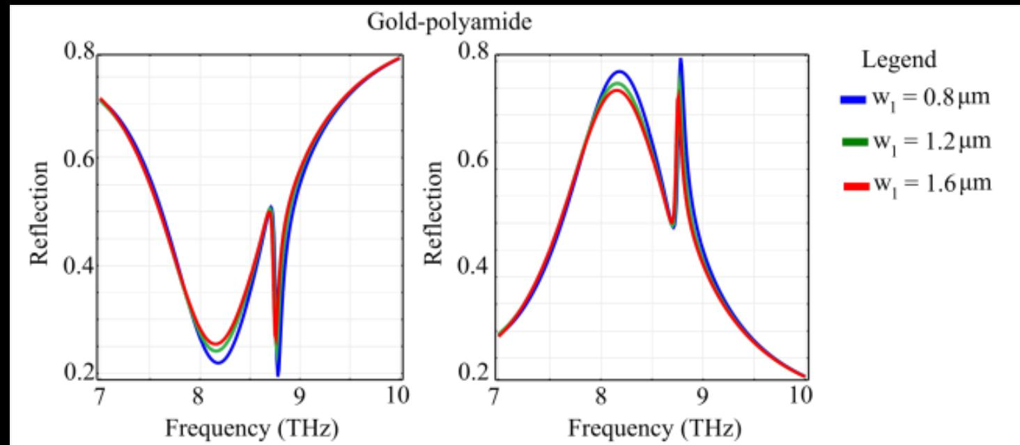
Spectral reflection and absorption of the gold-polyamide metasurface configuration, under variation of the thickness of the top rod  $w_1$ .
