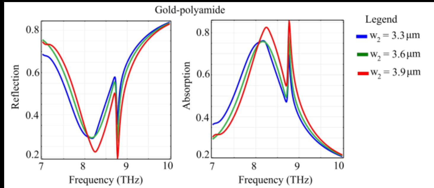
Spectral reflection and absorption of the gold-polyamide metasurface configuration under variation of the thickness of the base rod  $w_2$ .
