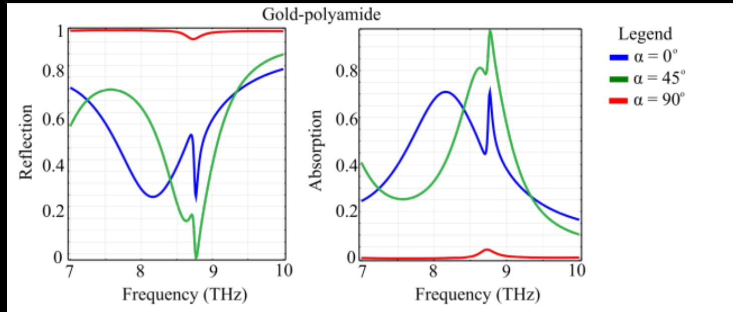
Spectral reflection and absorption of the gold-polyamide metasurface configuration under variation of the input linear polarization angle.
