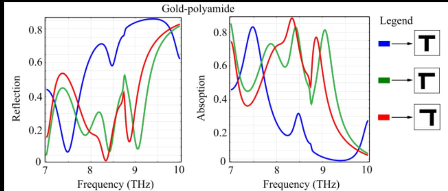
Spectral reflection and absorption of the gold-polyamide metasurface configuration, under variation of the relative coordinates of the base rod with respect to the top rod
