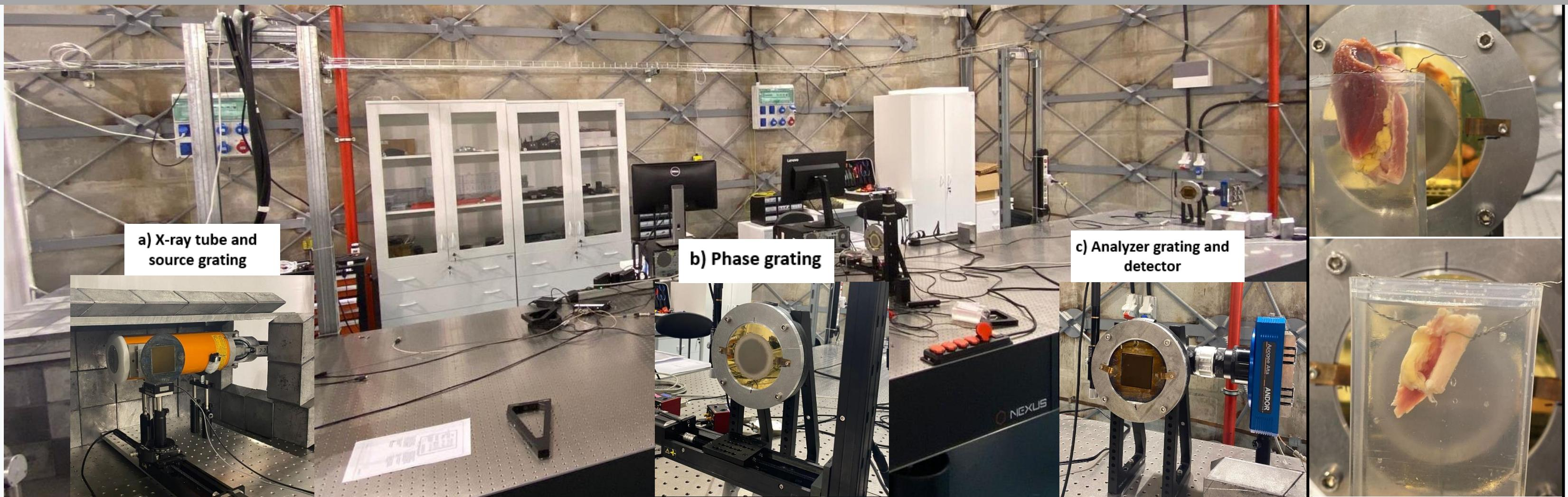
**5.66 m Long Talbot-Lau Interferometer, consisting of
