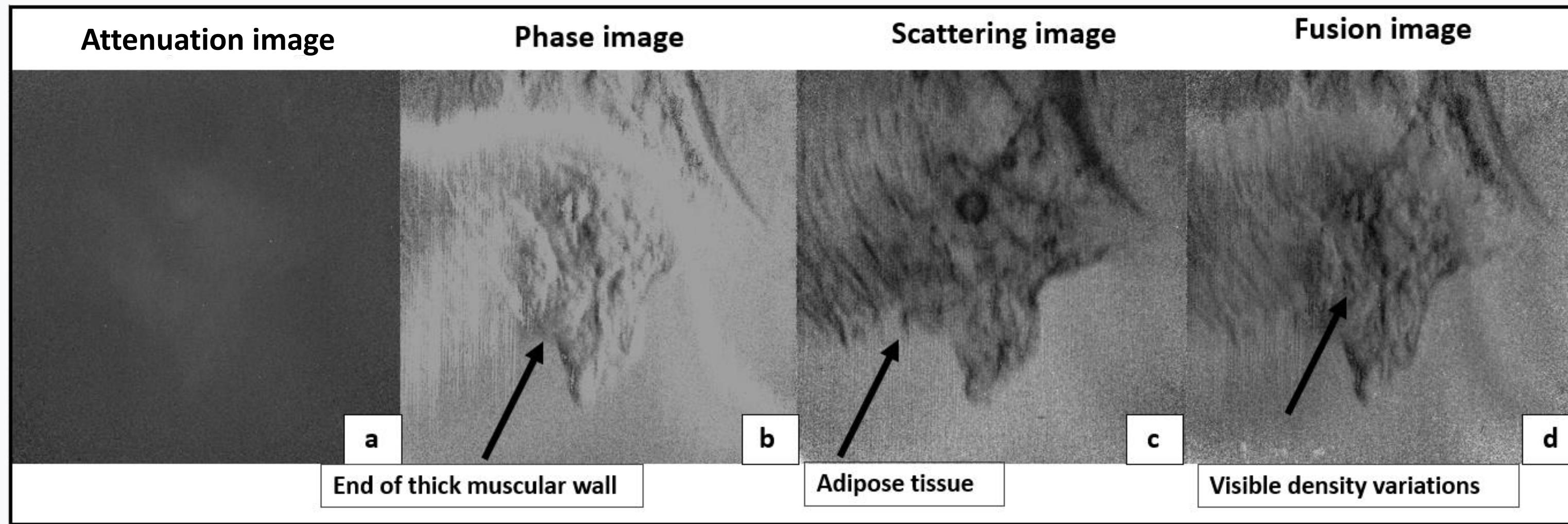
Experimental results for a chicken gizzard. a. attenuation image; b. differential phase contrast image; c. scattering image; d. fusion image (with the weighting constants set as follows:  $w_{att} = 1$ ,  $w_{phase} = 3$ , and  $w_{scatt} = 6$ )
