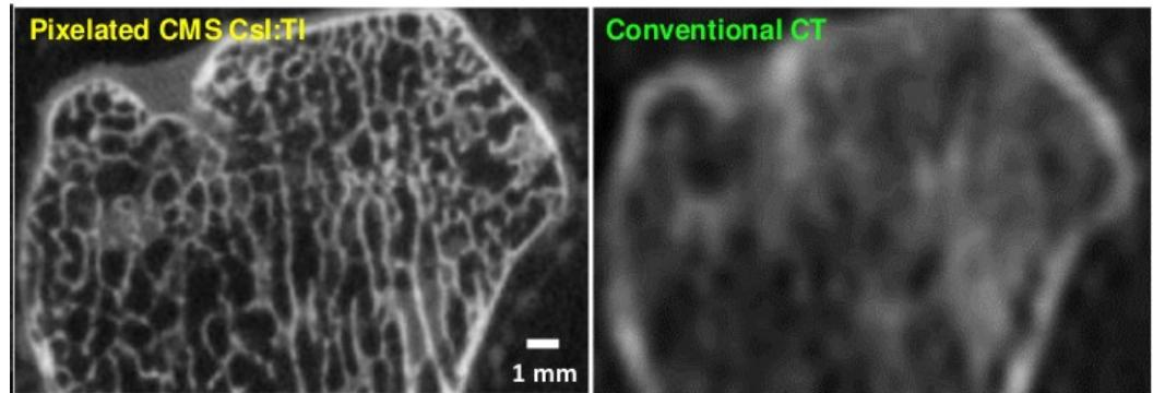
Images of a bone obtained using the CBCT based on pixelated CsI:Tl and conventional CT (for illustrative purposes only).
