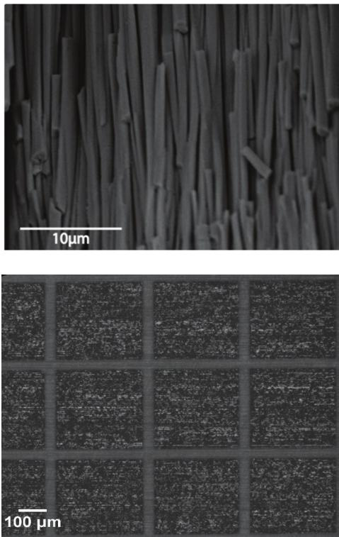
L. K. Jambi et al, *Comparison of columnar and pixelated scintillators*
