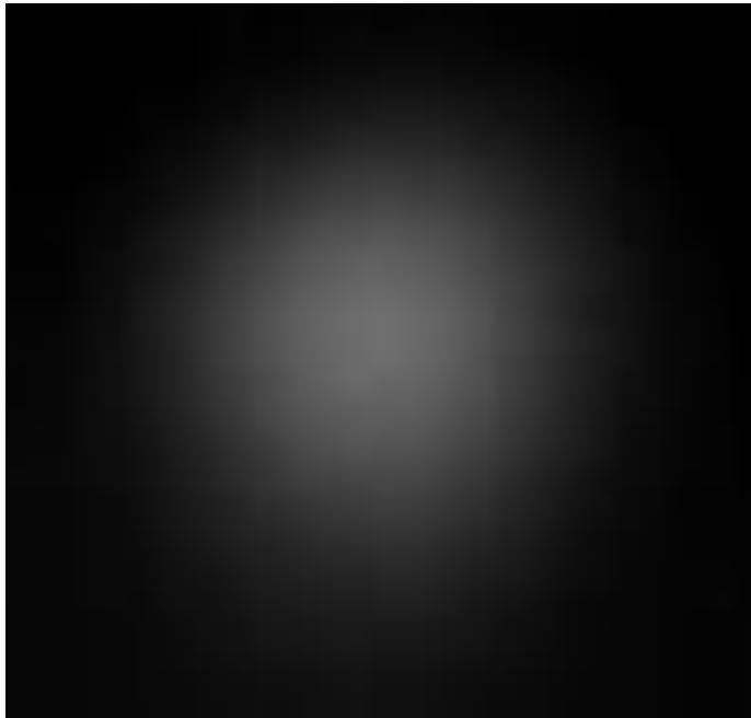
Spot size: 106.95  $\mu\text{m} \times 106.95 \mu\text{m}$
