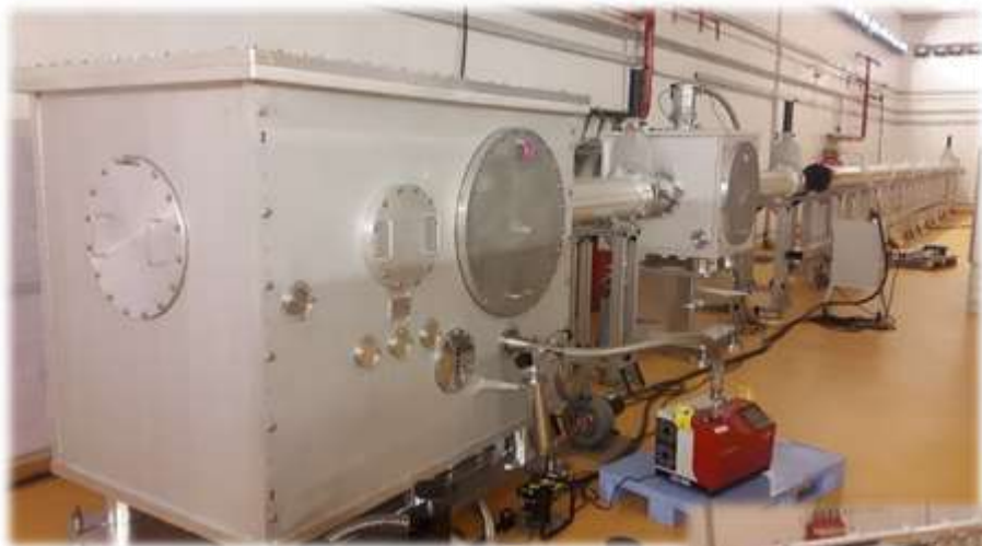
1PW beamline to E1-E6 Under vacuum leak tests.
