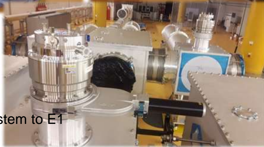
1PW beamline to E1-E6 Under vacuum leak tests.
